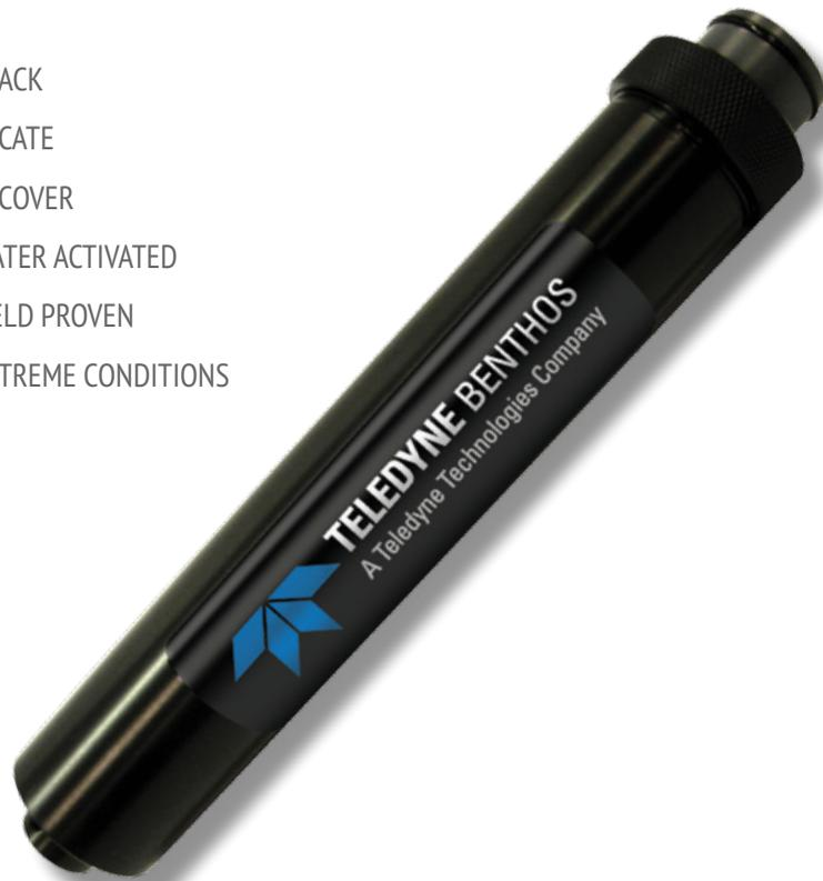
**Pingers** are used to mark underwater equipment or locations. They are generally about the size of a flashlight and can be attached to any mooring. The unit pings continuously when in the water. To recover a mooring, a diver or ROV is sent with a device to “listen” for, and home-in on, the pinger sound.
