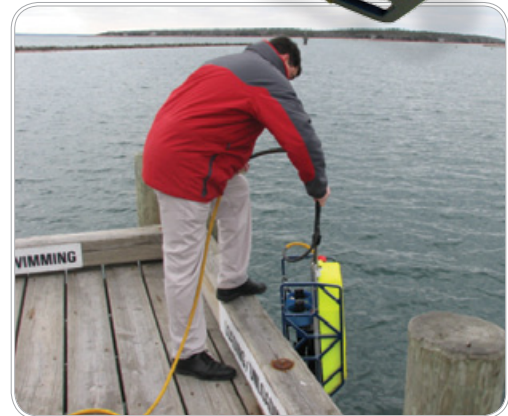
The MiniROVER is easily deployed and recovered by one person.
