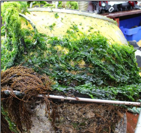
Fouling after fourteen weeks at sea.
