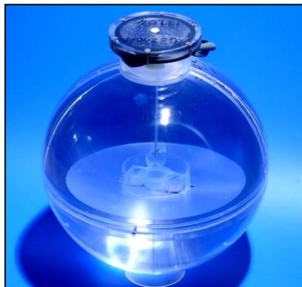
The Datawell stabilized platform sensor
