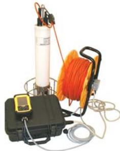
□ **MANUAL PORTABLE WINCH.** Includes 2-way or 5-way slip ring and it can hold up to 350 m of 5 mm polyurethane jacketed armoured cable or 100 m of 8.3 mm polyurethane multi-conductor shielded cable.
